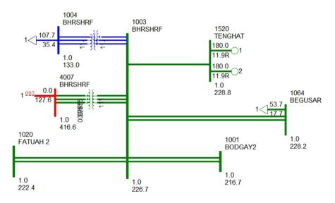
At 08:30 hrs, total power interruption occurred at Biharshariff (BSPTCL) 220/132/33kV S/s due to B-N fault on 220kV Biharshariff- Begusarai-I and subsequent tripping of 220kV Biharshariff-Begusarai-II along with 400/220kV,315 MVA ICT-I,II & III at Biharshariff (PGCIL) on operation of E/F back up overcurrent protection respectively. The following elements were tripped:
