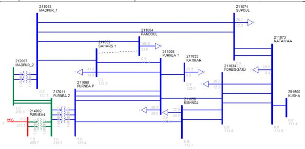
From SCADA data recorded at ERLDC it is observed that coincident with tripping of 132kV Purnea(PG) – Purnea(B) T/C, power flow through 220kV New Purnea-Madhepura D/C also became zero. Power supply to Madhepura and Sonebarsa also failed.
