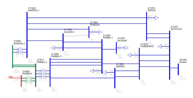
At 06:01 hrs, all 220/132kV, 100 MVA ATR-I, II & III tripped at Madhepura on operation of REF protection from 220kV side. However it is suspected that after tripping of above mentioned ATRs at Madhepura local load at Supaul, Phoolpras, Katiya & Nepal were catered through 132kV Purnea (PG)- Kishanganj & 132kV Purnea(B)- Forbisgunj S/c, which caused the tripping of the both 132kV
