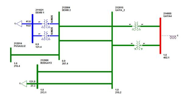
In 39<sup>th</sup> PCC, it was felt that N-1 security criterion is not satisfied at 400kV Gaya S/s and advised Powergrid to augment the 315 MVA ICT-II with 500 MVA capacity.
