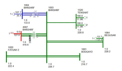
At 08:30 hrs, total power interruption occurred at Biharshariff (BSPTCL) 220/132/33kV S/s due to B-N fault on 220kV Biharshariff- Begusarai-I and subsequent tripping of 220kV Biharshariff-Begusarai-II along with 400/220kV,315 MVA ICT-I,II & III at Biharshariff (PGCIL) on operation of E/F back up overcurrent protection respectively. The following elements were tripped:
