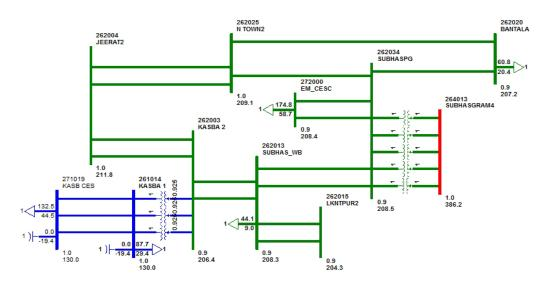
After tripping of 220kV Subhasgram(PG)-Subhasgram (WB) D/c and 220kV Jeerat-Kasba D/c lines, part of WBSETCL network along with CESC system got isolated from the ER grid and around 180 MW power was being exported to the part of WBSETCL network from CESC's EM Substation through 132 KV EMSS (CESC) – Kasba (WBSETCL) circuits.
