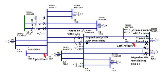
WBSETCL informed that there was a C ph-N fault (close to Jeerat end) in 132kV Jeerat-Mohispota line (under construction), which was idle charged from Jeerat end. Jeerat end failed to clear the fault. As a result the following lines tripped:
