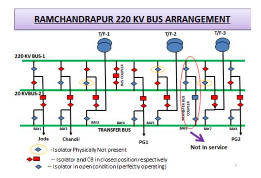
From the SLD it can be seen that many of the isolator are physically not present or nonoperational which causing constraints in system operation.
