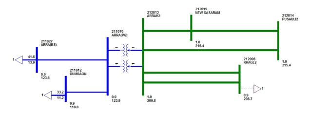
At 11:50 hrs, 220 kV Nandokhar – Arrah S/C tripped from Nandokhar end due to high voltage at Nandokhar.
