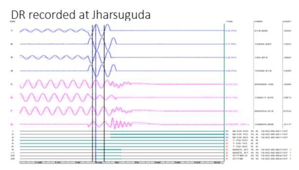
Pre-fault current: 55-60A in each phase; Post fault current: 200 A in R & B phases and 10.5 kA in Y phase
