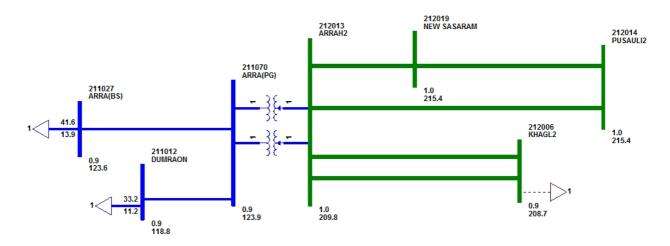
At 09:20 hrs tripping of 132 kV Arrah(PG) – Arrah(BSPTCL) S/C line tripped due to R-N fault (Z-I from PG end) during heavy storm resulted load loss at radially fed areas. Arrah(BSPTCL) did not trip as no other source is connected.
