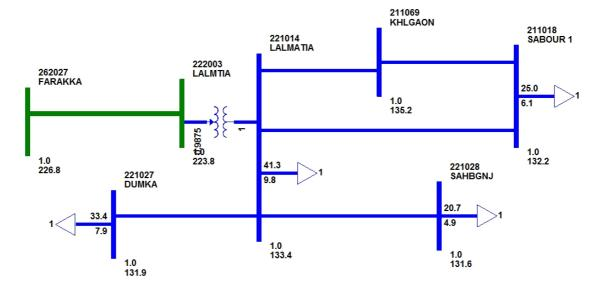
At 16:39 hrs 220 kV Farakka Lalmatia S/C line tripped from Farakka end on O/C E/F protection F/C 4.68 kA in B phase at Farakka.
