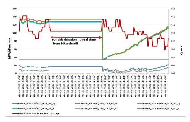
Event 3: 400/220 kV ICT I and II tripped at Patna at 18:53 Hrs on 03.07.2017
