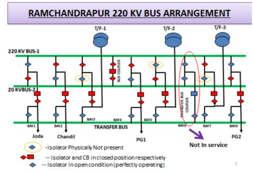
From the SLD it can be seen that many of the isolator are physically not present or nonoperational which causing constraints in system operation.
