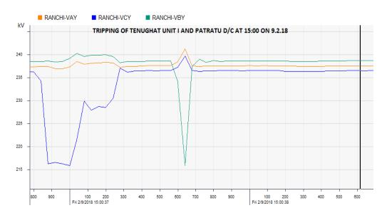
In PMU data, two faults have been observed. First fault was in B phase at 15:00:36.800 hrs which was cleared in 500 ms. 300 ms after clearing the first fault, another fault was observed in Y phase which was cleared within 100 ms.
