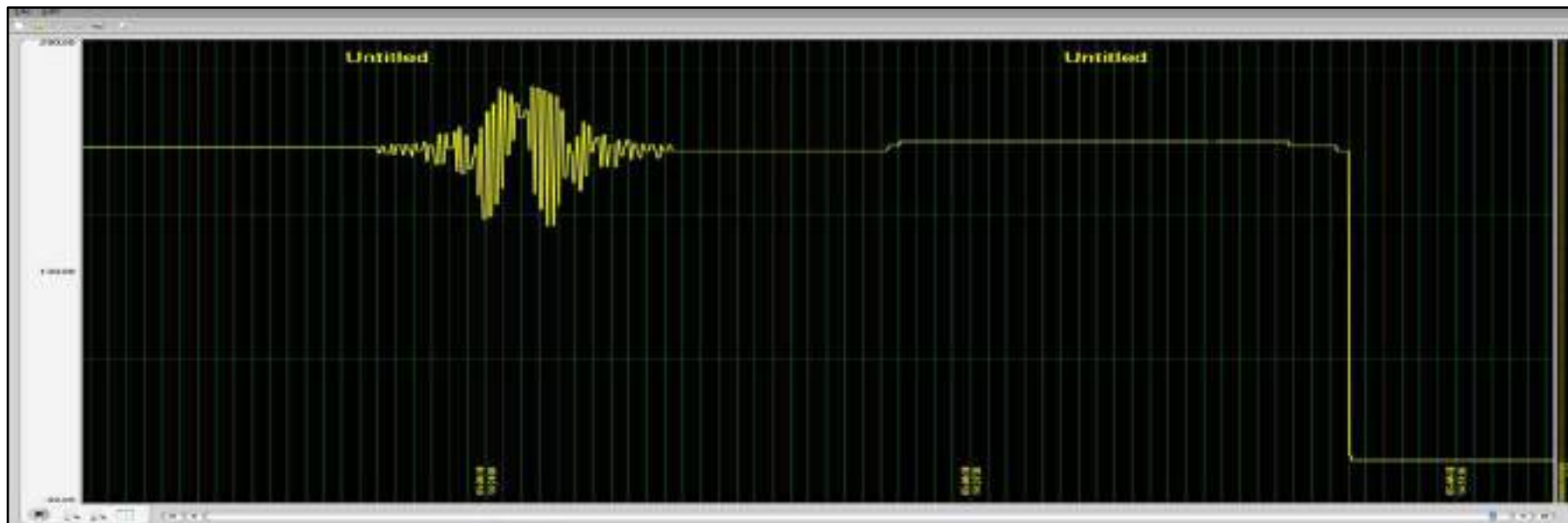
Fig : MW variation of the Sagardighi unit 4 and its subsequent tripping observed from ERLDC SCADA for 5 th April' 18.
