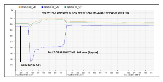
This led to blackout of 400 kV Tala substation causing loss of 447 MW generation. The tripping of 400 kV Malbase-Tala circuit is not shared with ERLDC as this circuit might also have tripped during the blackout of Tala generation.
