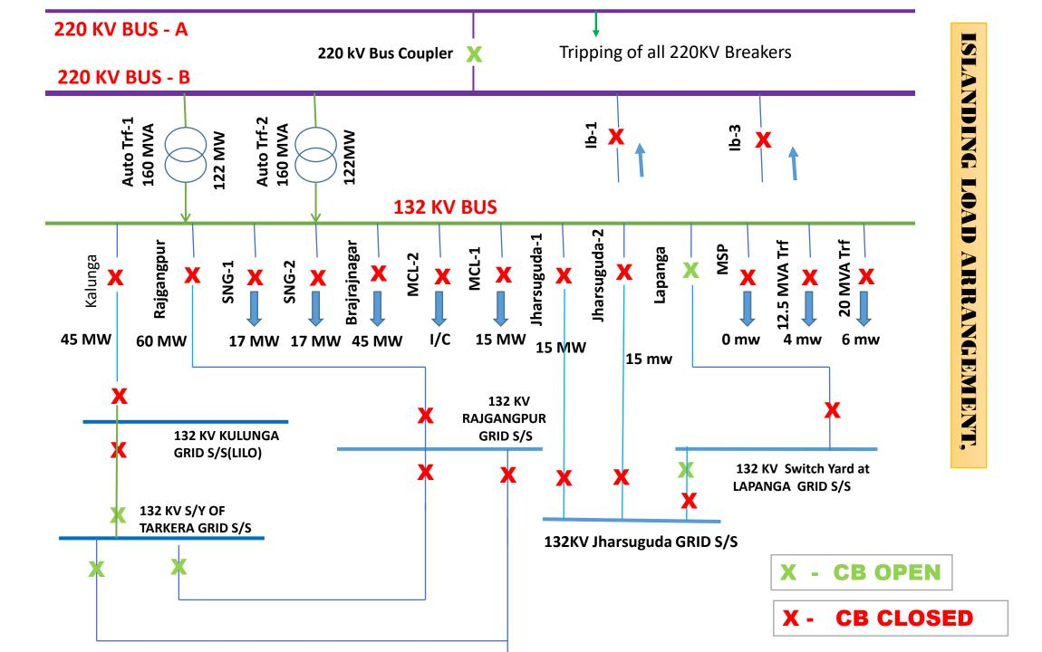
SCHEMATIC DRAWING OF ISLANDING RELAY INSTALLED IN B/C PANEL FOR TRIPPING OF DIFFERENT FEEDERS AT BUDHIPADAR GRID S/S.
