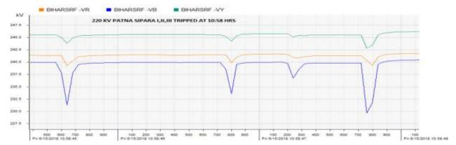
As per PMU data, multiple faults have been seen in B phase around 10:58 hrs which got cleared within 100 ms.
