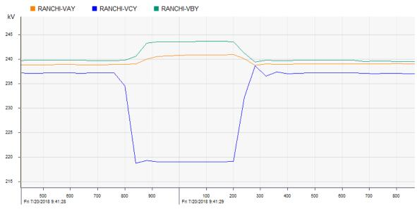
Figure 4: 400 kV Bus voltage at Ranchi at 09:41:28:00 hrs
