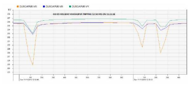
PMU observation at Durgapur end for the fault at 12:50 hrs
