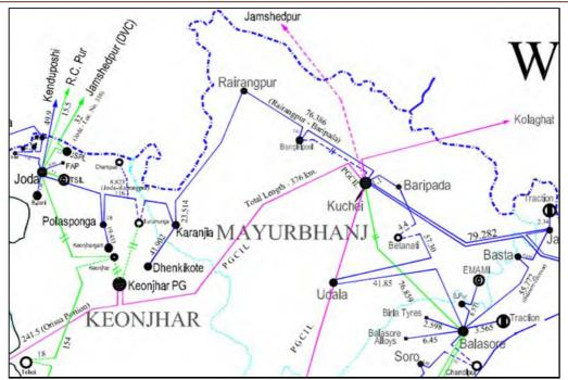
Hence, OPTCL has requested for allotment of a new 132 kV Bay at Kuchei to limit the line loading (Kuchei–Bangiriposi portion) as well as to meet the n-1 contingency. OPTCL plans to draw a new 132kV S/c line from Kuchei to Bangiriposi as intra-state scheme.
