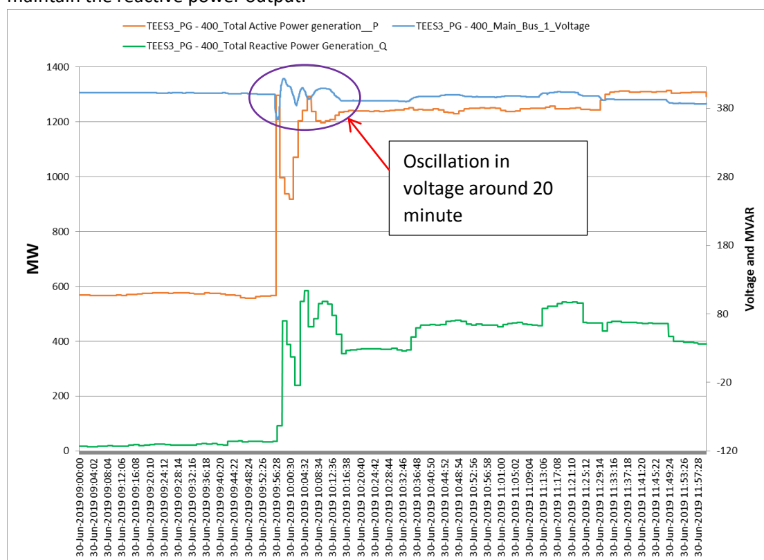
Figure 9: Active Reactive generation of Teesta III and Teesta III Bus voltage
