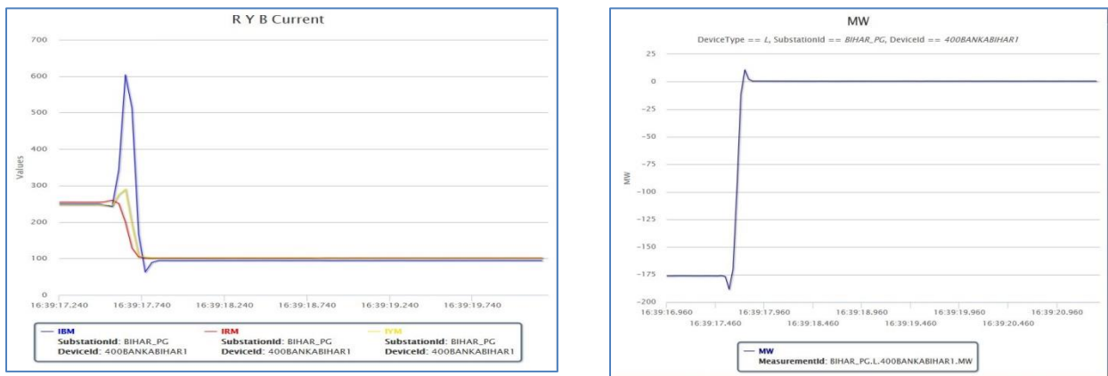
Figure 3: Three phase current and MW power flow measured for 400 kV Biharshariff - Banka - I at Biharshariff end shows the non - auto-reclose operation of 400 kV Biharshariff Banka – I
