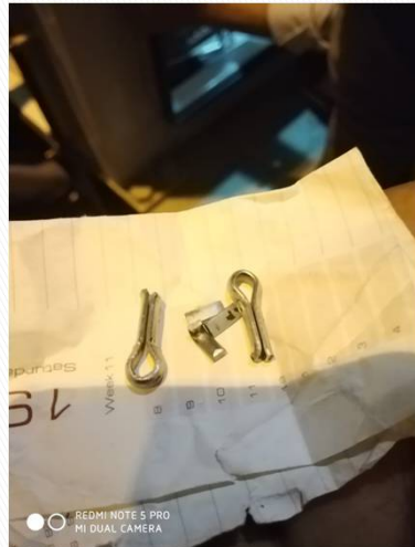
BROKEN COTTER PIN
