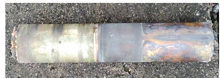
Dislocation of spindle due to damaged lock
