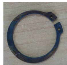
Dislocation of spindle due to damaged lock
