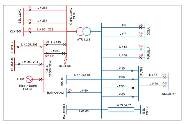
It is suspected that fault was at 220 kV bus at CTPS – A s/s. As Bus bar protection was not in service, 220 kV feeders and 220/132 kV ICTs at CTPS – A tripped from remote end in back up protection.
