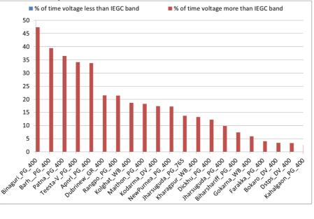
It can be seen that many of the high voltage nodes such as Barh, APNRL, Kolaghat, Koderma etc. are generator nodes or close to generator node. As generators are not absorbing sufficient MVAr as per their capability curve is one of the reason for this sustained high voltage.
