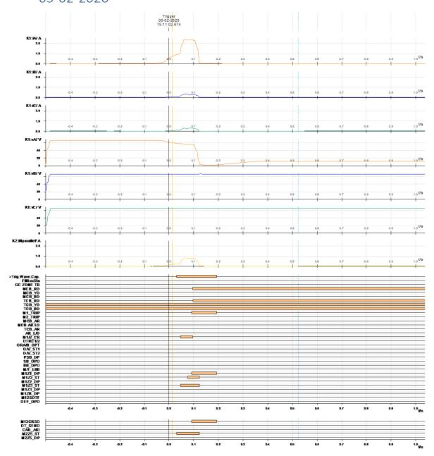
Issue: Post fault DR time window less than 1.1 sec; A/R operation not properly captured; Y and B phase T CB remained open prior to the tripping;
