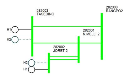
In 88<sup>th</sup> PCC meeting ERLDC informed that there was a B-N fault in 220kV New Melli-Jorethang line -I and Jorethang end tripped on zone 1. The fault got cleared within 100 ms. Reason for tripping of 220 kV New Melli-Tashiding S/C, 220 kV-Tashiding-Rangpo S/C lines needed explanation.
