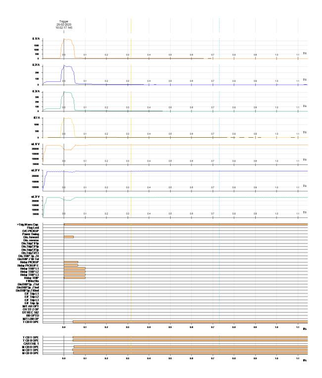
Issue: DR at Sagardighi end is not time synchronized; Time of both DR shared is different from tripping time. It is reported Z-II was triggered from Sagardighi end. Reason of tripping is not recorded.
