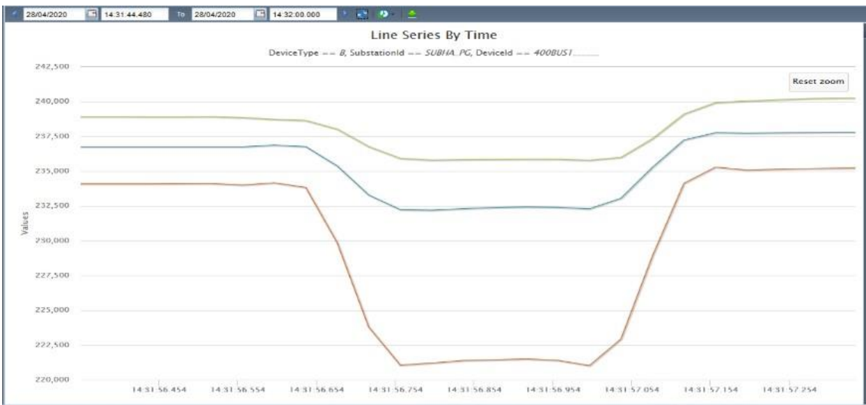
Figure 2: Three phase voltage recorded at Subhasgram PMU at the time of the disturbance shows delayed clearance of R phase to earth fault. Fault clearing time is around 300 ms.
