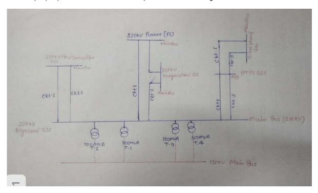
At 11:01 hrs 220 kV Biharshariff-Barauni D/C tripped from Biharshariff end on B-Phase to earth fault with delayed fault clearance observed in PMU. At the same time 220 KV Barauni-Begusari-1 tripped in zone-2 from Barauni end.
