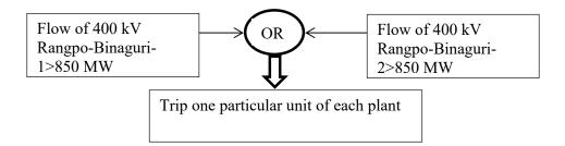
In 94<sup>th</sup> PCC, ERLDC explained that flow of 400 kV Rangpo-Binaguri-1 and II is to be measured and if the power flow greater than 850 MW in any one line then SPS signal would be generated and issue trip command to one unit of each plant i.e. Teesta III, Dikchu, Jorethang and Tashiding HEP.
