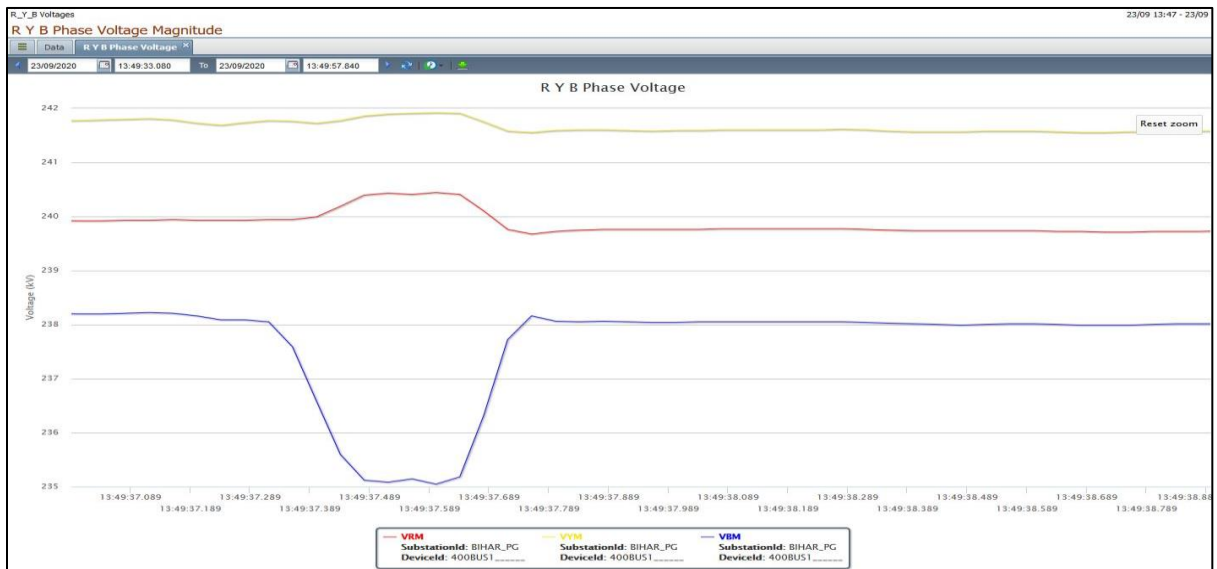
Figure 4: Three phase PMU recorded at 13:49 hrs at Biharshariff shows the existence of B phase to earth fault. The fault clearing time was less than 160 ms.
