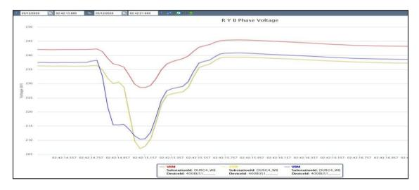
As per Durapur PMU, fault was in R, Y and B phase at 02:42 hrs. Around 30 kV dip has been observed in Y and B phase voltage while 12 kV dip in R phase is recorded in the PMU. The fault clearing time was around 800 ms.
