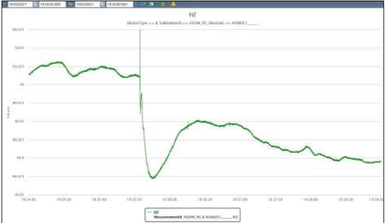
Figure 6: Frequency variation captured at Kishangunj PMU during the event. Rest of the grid frequency dropped from 50.01 Hz to 49.87 Hz. Later it stabilized to 49.95 Hz.
