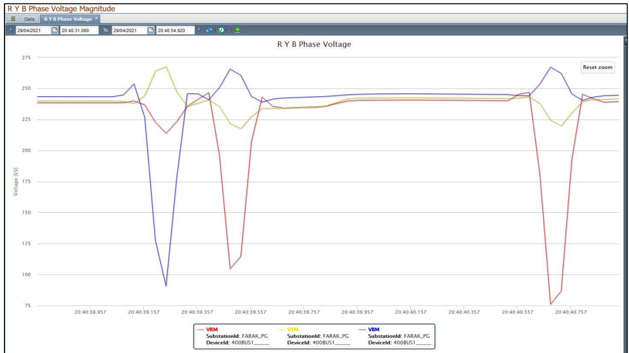
Figure 2: Three phase voltage measured by Farakka PMU shows the existence of one B phase to earth fault and one persistent R phase to earth fault at the time of the event.
