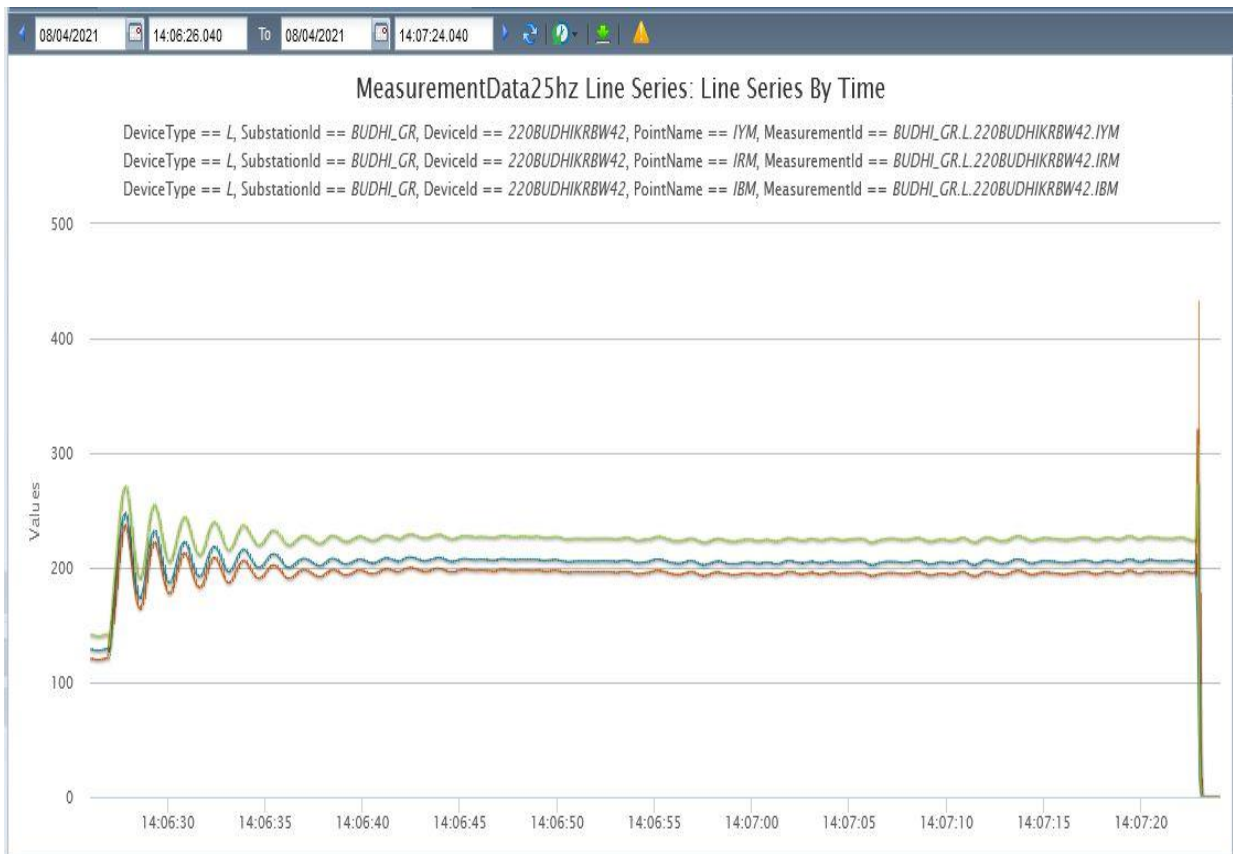
Figure 13: 220 kV Budhipadar-Korba East 2 Line current indicating R phase fault and its tripping on bus bar protection for 220 kV Bus 1 on which it was connected.
