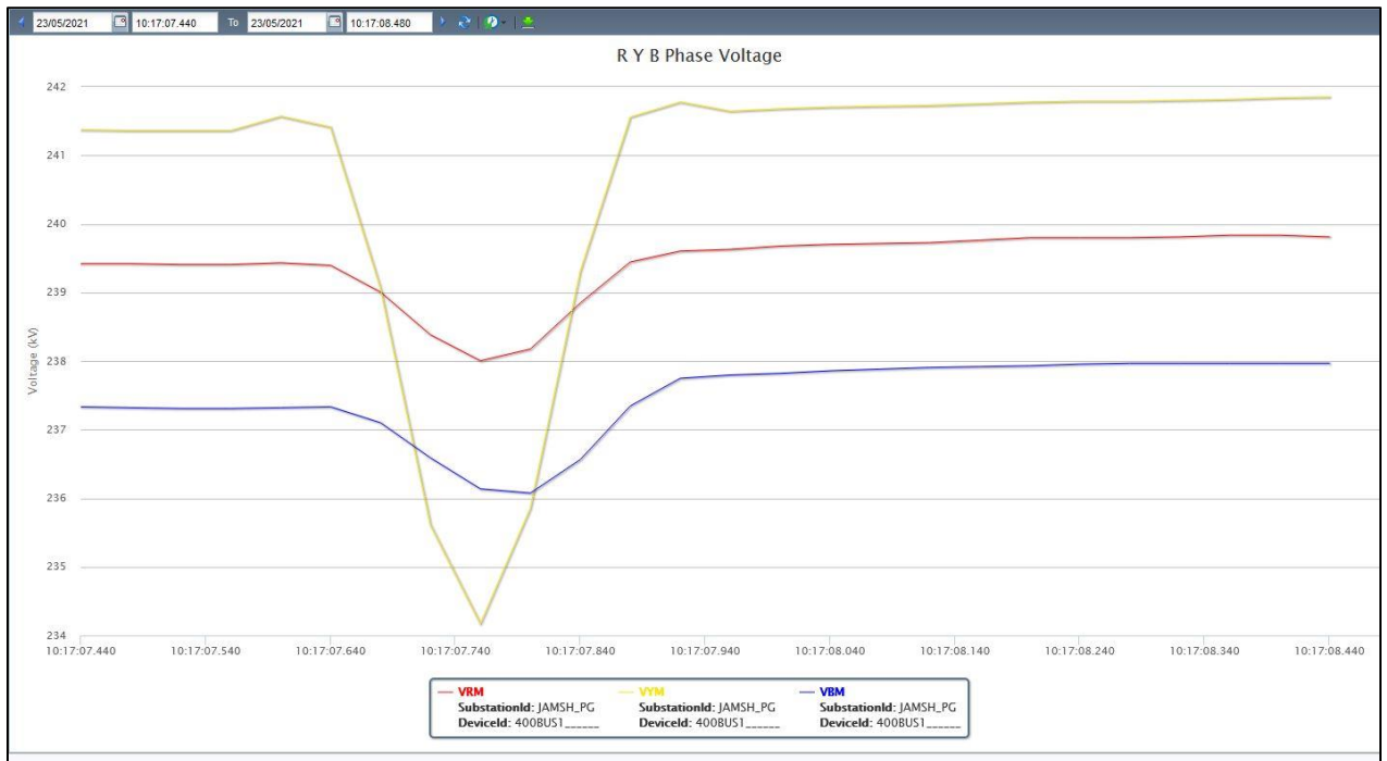
Figure 3: Three phase bus voltage captured by 400 kV Jamshedpur PMU shows existence of Y phase to earth fault at 10:17 hrs. Around 7 kV dip has been observed in Y phase voltage at Jamshedpur PMU. Fault clearing time was less than 100 ms.
