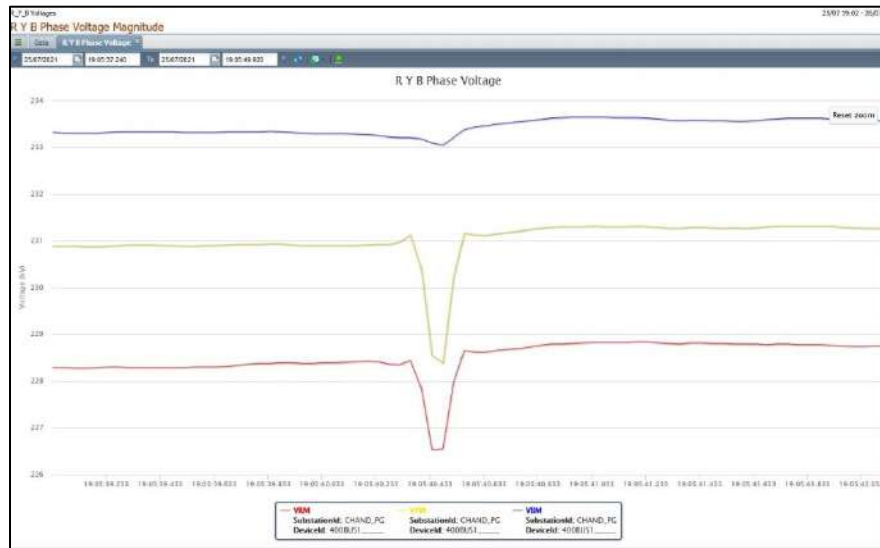
Figure 3: PMU captured at Chandauti shows 3kV dip in R and Y phases indicating fault in R-Y phases.
