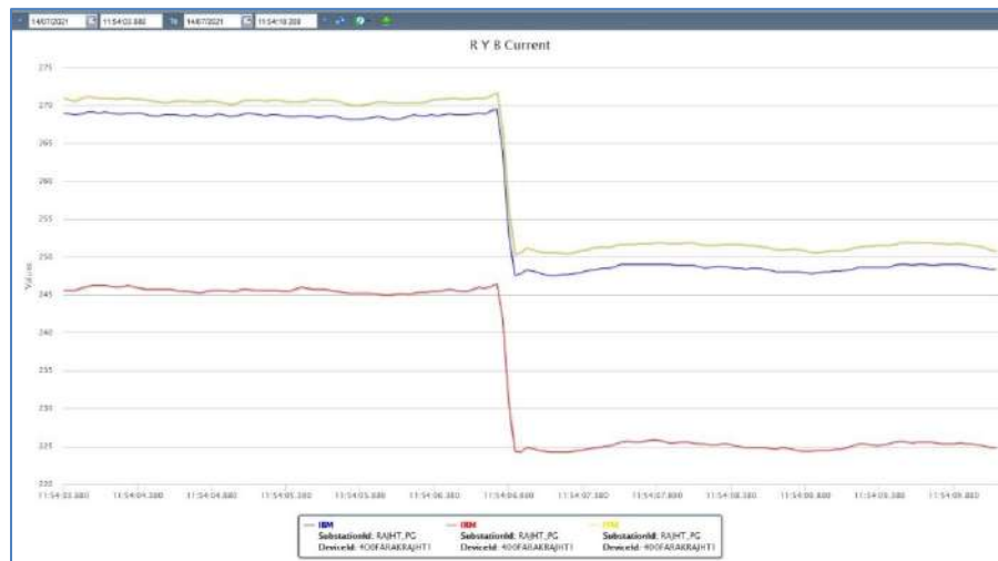
Figure 4: PMU captured at Rajarhat shows no fault and 20 kV dip in voltage is observed in all phases.
