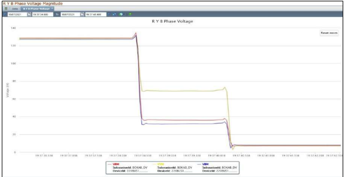
Figure 3: PMU captured at Bokaro shows fault was cleared in around 1.5 seconds after first dip
