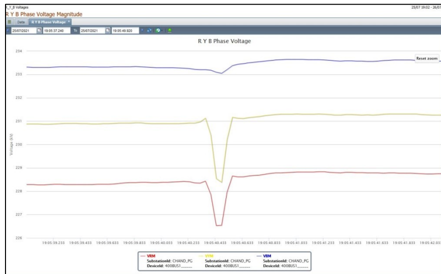
Figure 3: PMU captured at Chandauti shows 3kV dip in R and Y phases indicating fault in R-Y phases.
