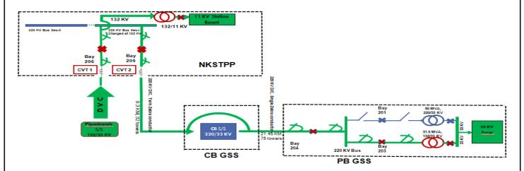
They requested for granting permission for charging of 220 kV D/C transmission line from NKSTPP to Pakri-Barawdih S/s via Chatti-Bariuati S/s as an interim mode at 132 kV Level.
