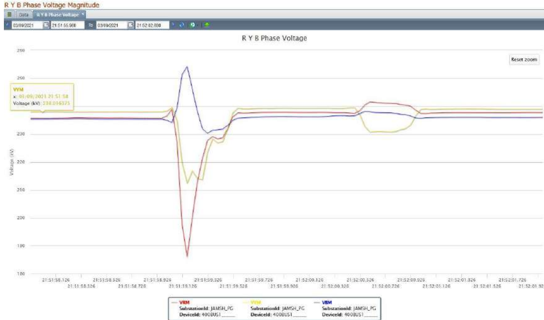
Figure 3: PMU snapshot of 400/220 kV Jamshedpur S/s
