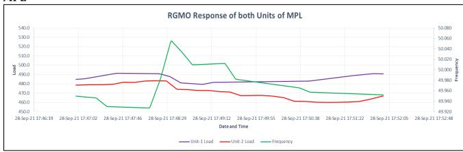
Maximum response observed: -11.2 MW for unit 1 and – 12.8 MW for unit 2.
