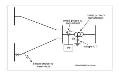
Following the DVC's practice the line DEF and Transformer DEF can be coordinated. The overall recommendation is as follows for the satge-1 setting:
