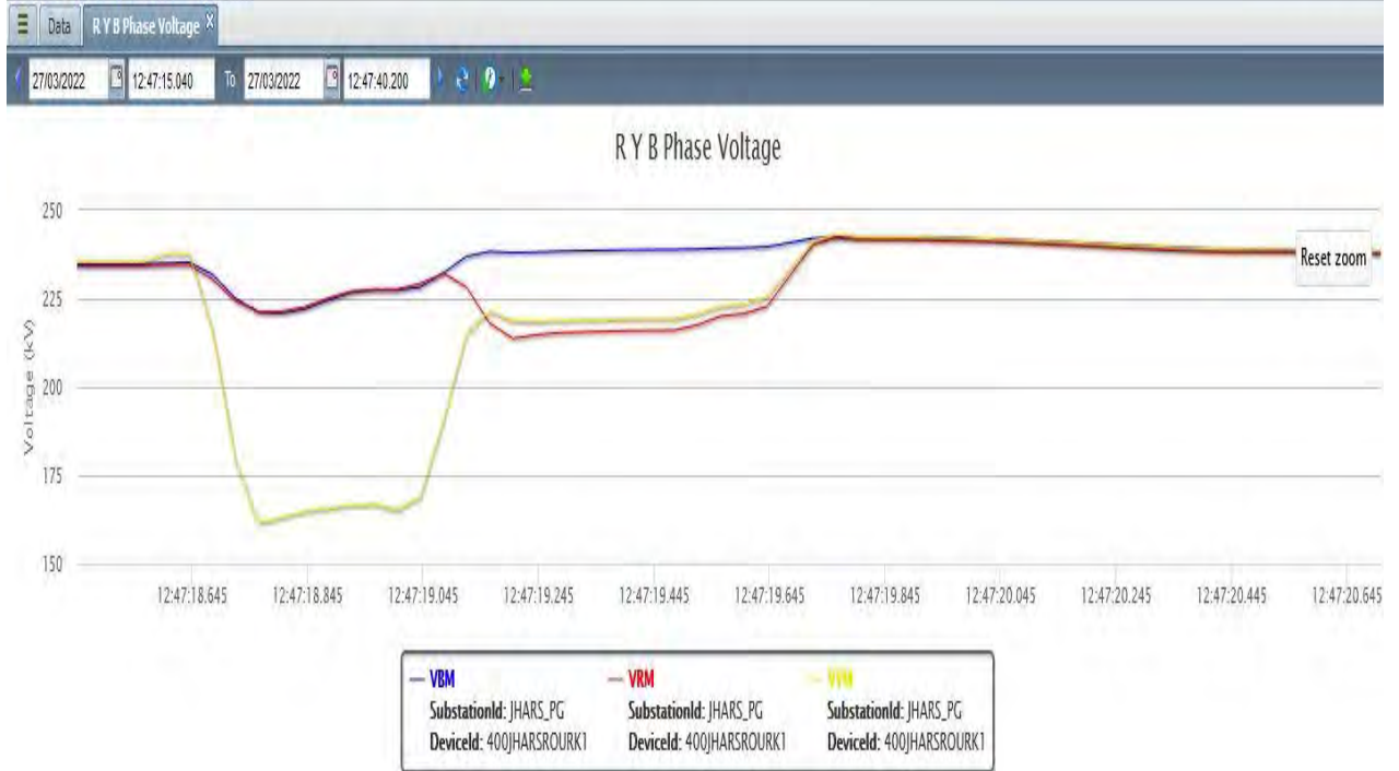
Figure 2: PMU voltage snapshot of 400/220 kV Jharsuguda S/s
