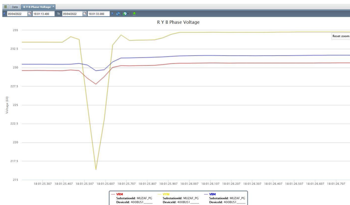
Figure 2: PMU voltage snapshot of 400/220 kV Muzzaferpur S/s
