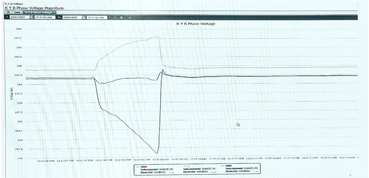
Figure 2: PMU voltage snapshot of 400/220/132 kV Rangpo S/s
