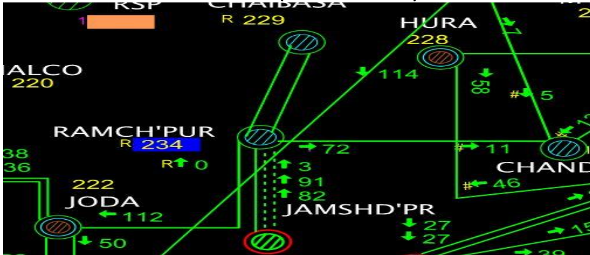
Figure 1: SCADA snapshot for of the system
