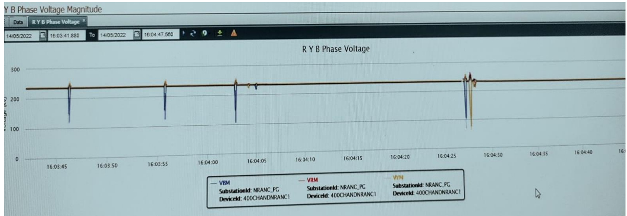
PMU Voltage snapshot of 400 kV New Ranchi S/s
