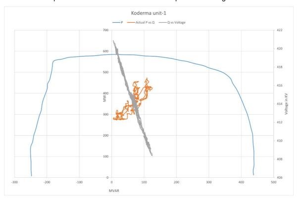
Therefore, Koderma power plant was requested to absorb MVAR as per their capability and maintain voltage well below 420 kV at Koderma bus so that all the nearby bus voltage remain within IEGC band. So all other generating stations are also requested to absorb MVAR at the time of high voltage to maintain the bus voltages within acceptable limit in view of upcoming winter season.
