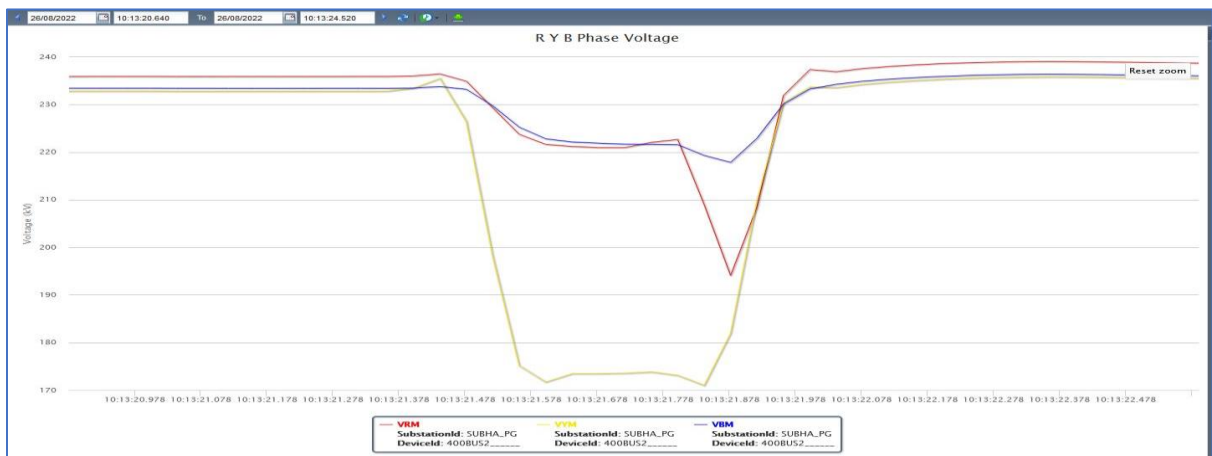
Figure 3: PMU Voltage snapshot of 400/220 kV Subhashgram S/s
