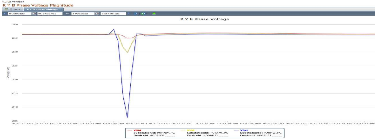
Figure 2: PMU Voltage snapshot of 400/220 kV New Purnea S/s
