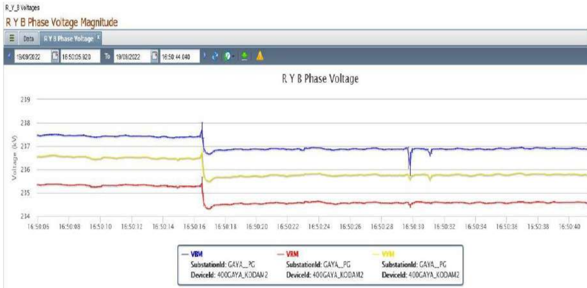
Figure 2: PMU Voltage snapshot of 765/400/220 kV Gaya S/s
