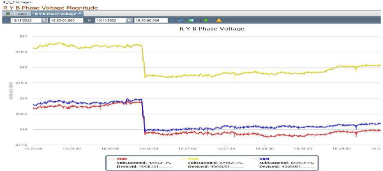
Figure 1: PMU Voltage snapshot of 400/220 kV Rangpo S/s at 16:26 Hrs
