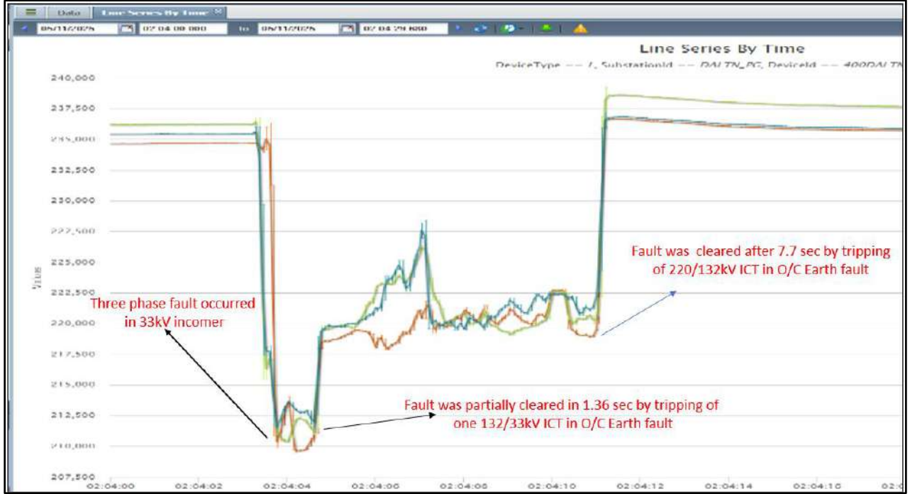
Figure 2: PMU plot at 400KV Daltonganj Sasaram line#1 Voltage during tripping of 132 kV system
