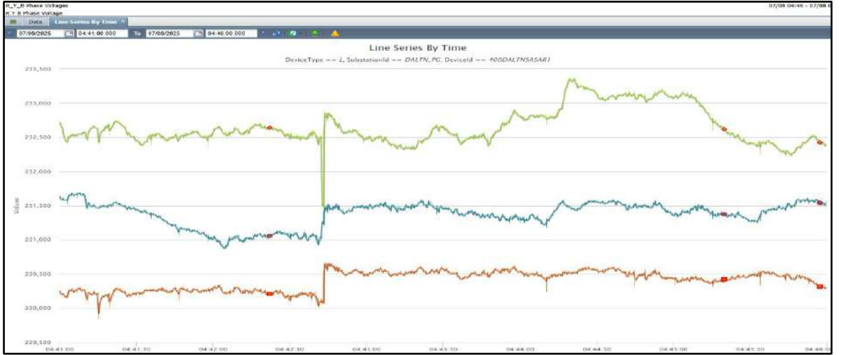
Figure 2: PMU of voltage at 220 kV Daltongaunj
