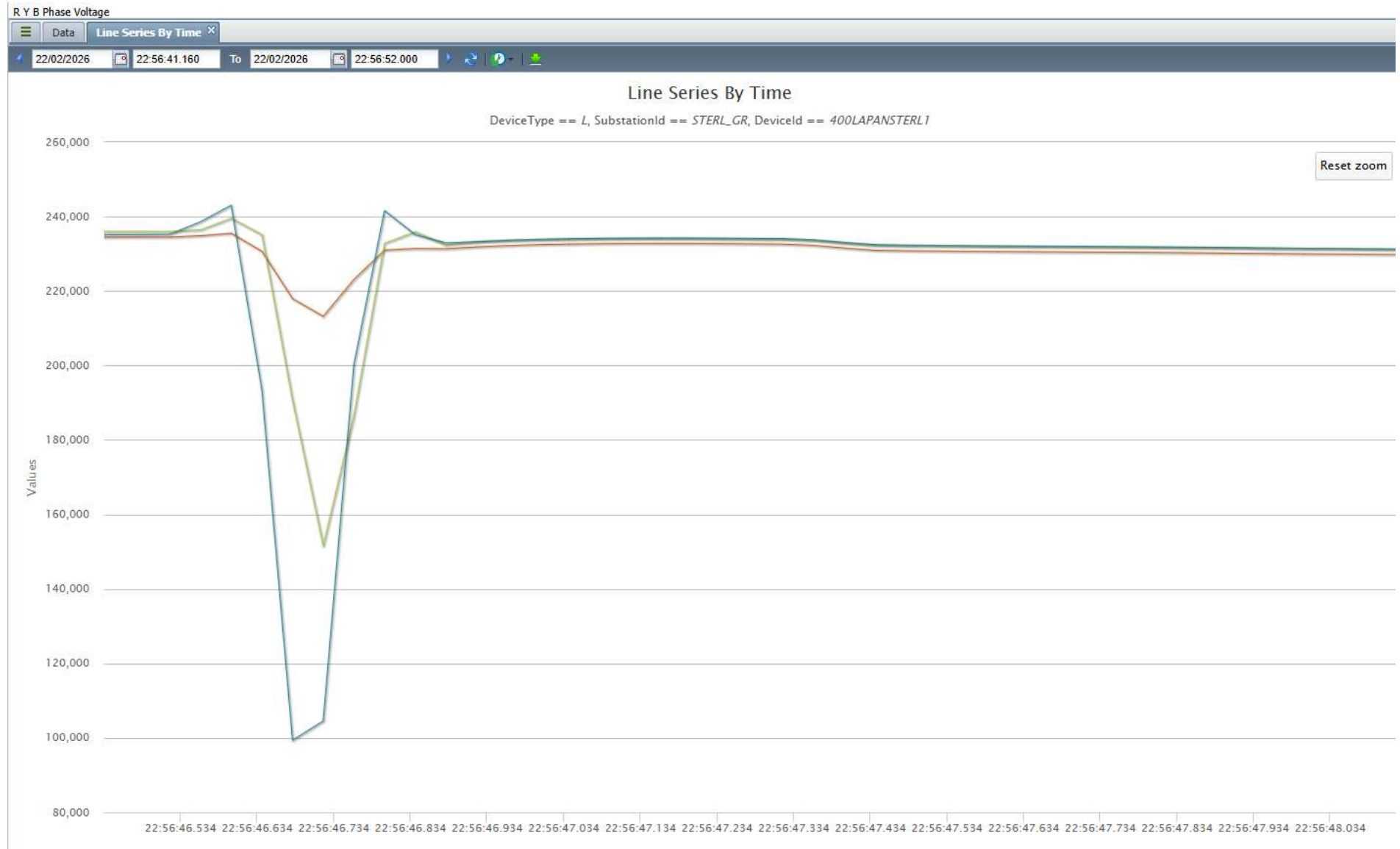
Line PMU voltage of Lapanga at Sterlite
