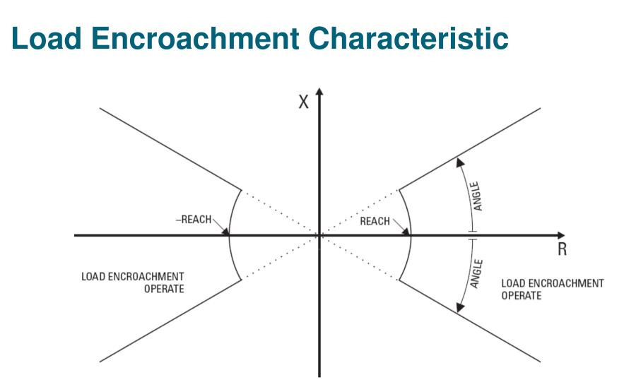
The load encroachment element responds to positive sequence voltage and current and can be used to block phase distance and phase overcurrent elements.
