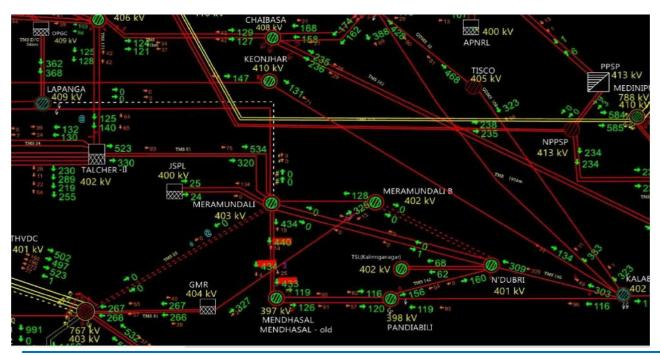
On 10th June at 17:27 hrs. during charging attempt of 400 kV Lapanga-Meramandali 1 from Lapanga end, all 400 kV Lines and 400/220 kV ICTs emanating from Lapanga along with 400 KV Lines from OPGC tripped. Due to absence of evacuation lines, only running unit of OPGC tripped resulting into loss of 580 MW generation. It is clearly evident that relays have not been properly coordinated in the said pocket.
