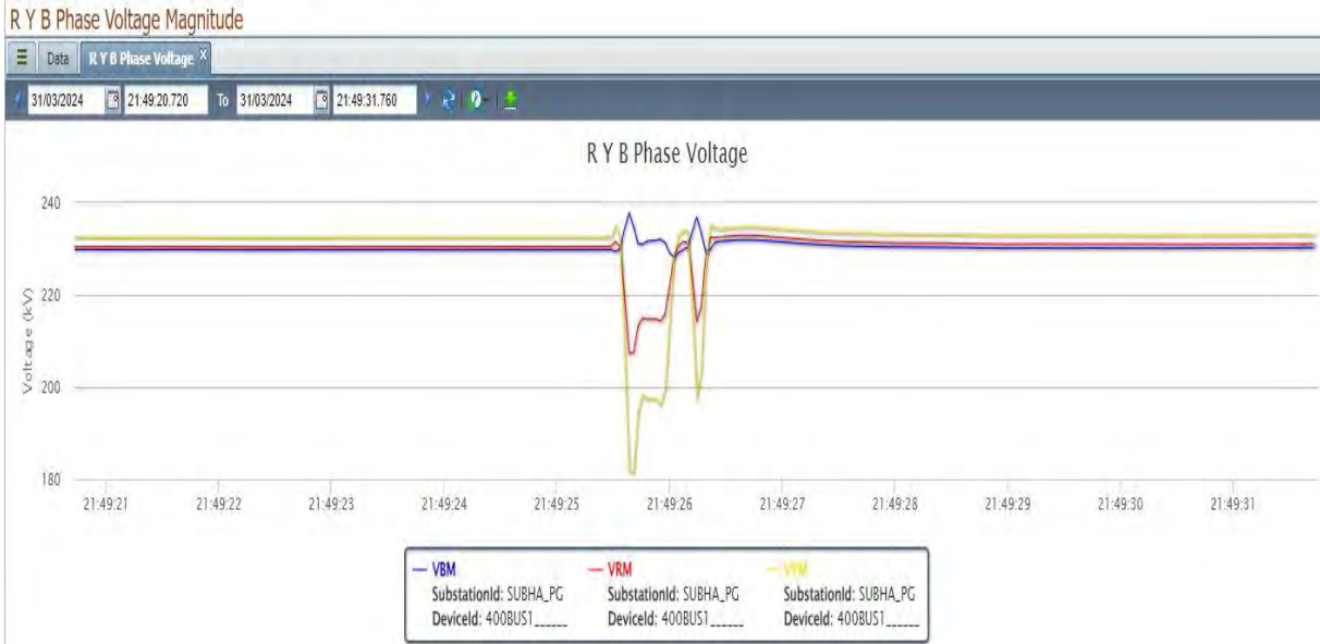
Figure 2: PMU Voltage snapshot of 400/220 kV Subhashgram S/S
