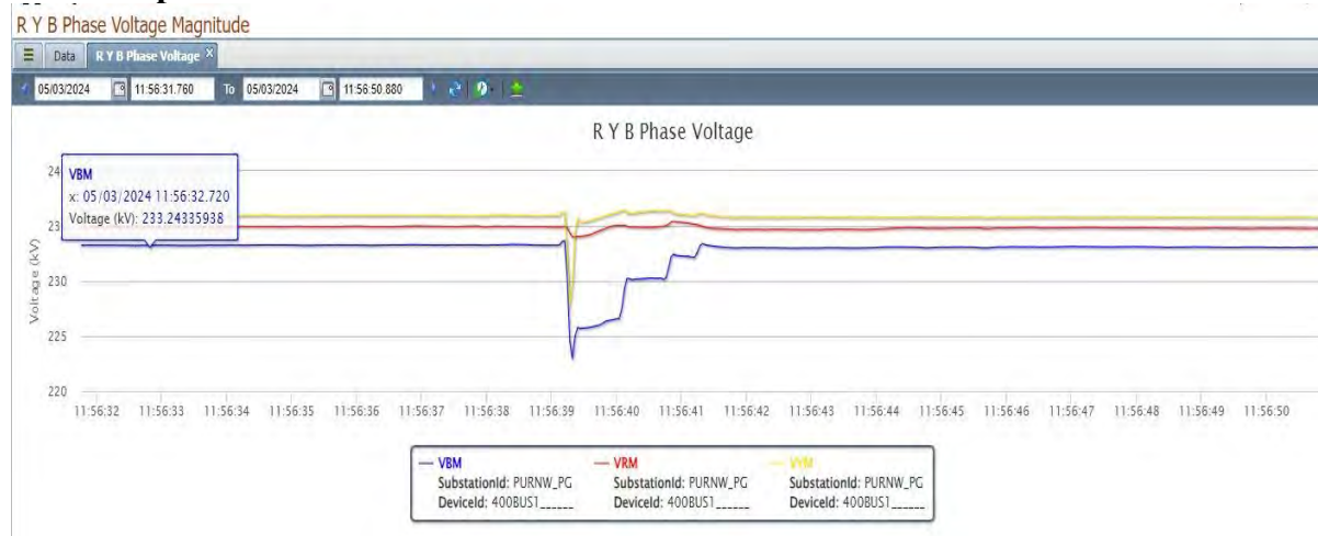
Figure 2: PMU Voltage snapshot of 400/220 kV New Purnea S/S
