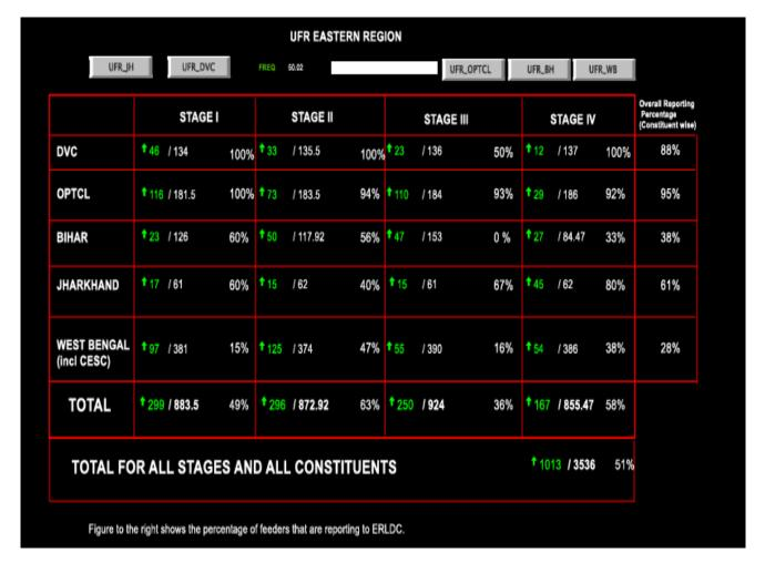
It is observed that 100% of UFR stage-1 feeders are not integrated (as on date) with the telemetry system of the few states. UFR feeder data integration may be prioritized for proper load visibility to get prepare for any greater contingency. State wise SCADA availability of UFR data enclosed at **Annexure B.2.6.2.1**
