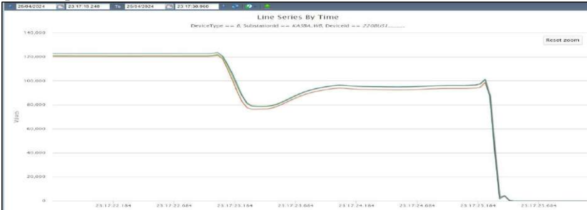
Figure 2: PMU Voltage snapshot of 220 kV Kasba S/S
